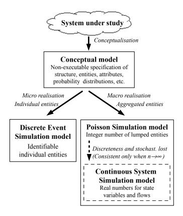
Figure 2. The relationships between System at study, Conceptual model, Discrete Event Simulation, Poisson Simulation and Continuous System Simulation.
