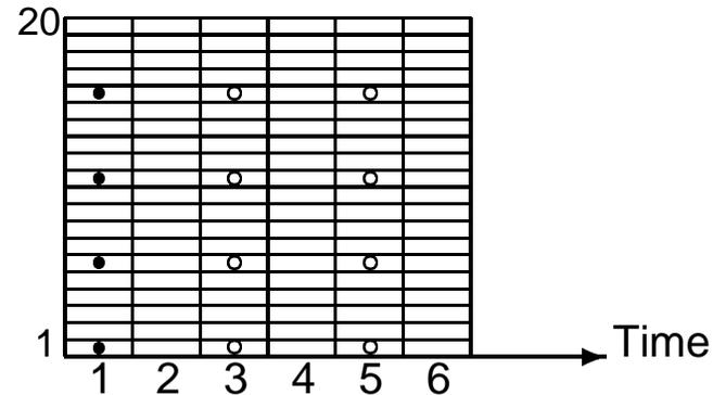
Figure 1: One of the time-frequency bins, containing 20 subcarriers with 6 symbols each. Known 4-QAM pilot symbols (black) and 4-QAM downlink control symbols (rings).
