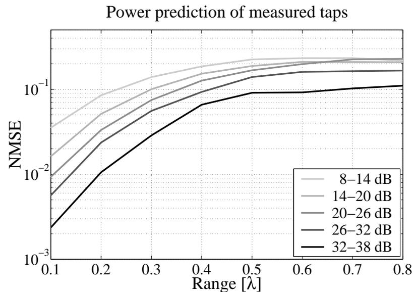
Median of the power prediction NMSE as function of the prediction horizon for cases with different estimation error power (CEER) on the regressors.
