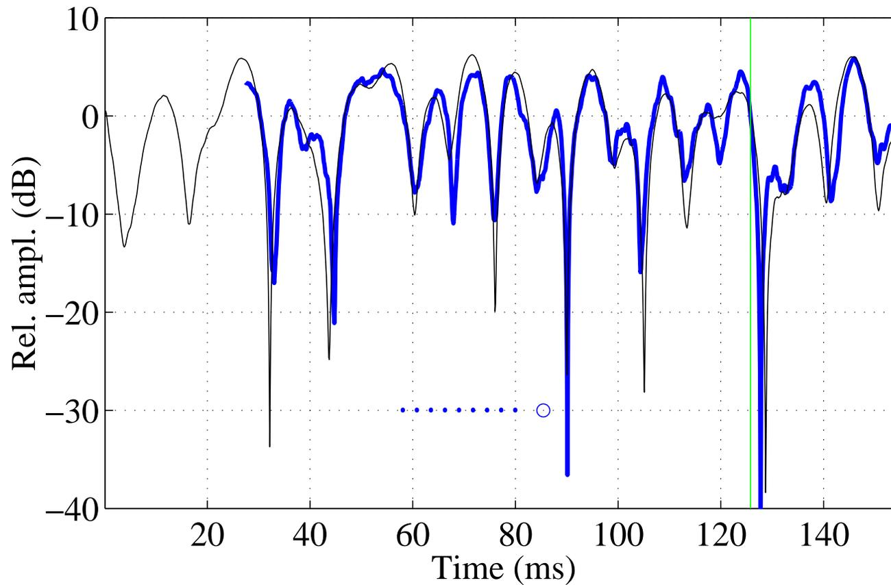
Predict the channel power (and interference power) over a horizon corresponding to 0.3 wavelengths (=2 ms at 2 GHz carrier and 100 km/h terminal velocity.)
