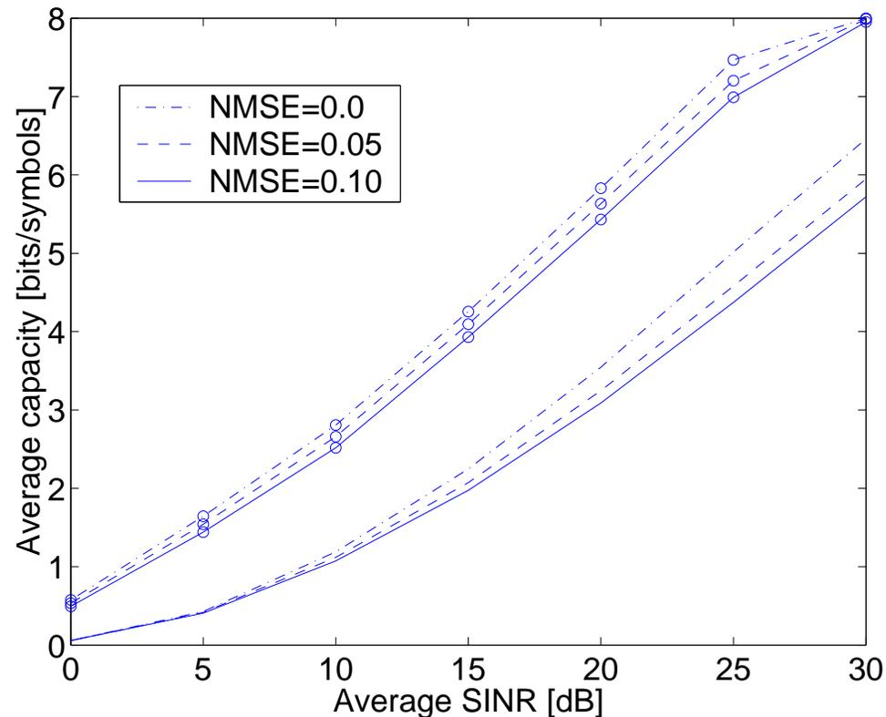
Average capacity as a function of the average SINR, equal for all users, with  $K = 1$  active users (lower curves) and  $K = 20$  terminals (upper curves with rings).
