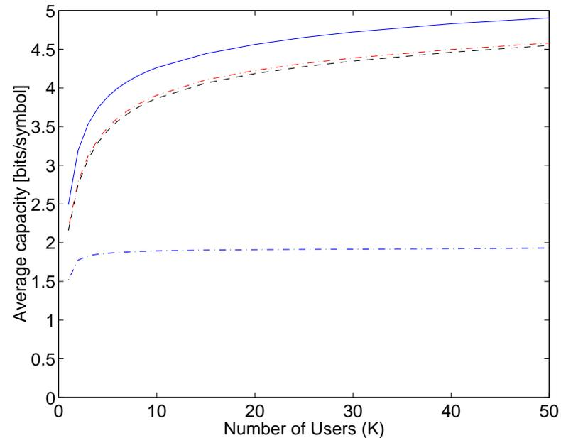
Spectral efficiency for average SINR 16B (same for all) when selecting the highest SINR out of  $K$  independent Rayleigh fading users. Solid: Perfect prediction. Dash-dotted: prediction NMSE 0.1, with optimized rate limits. Dashed: prediction NMSE with rate limits adjusted for perfect prediction. Lower dash-dotted: NMSE 0.495. **Conclusions:**
