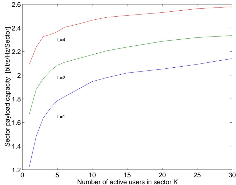
Figure 2: Estimated sector capacity with Rayleigh fading (no shadow fading). Two zones, limit 0.7 of radius (**reuse 1.73**). **OFDM-overhead factor 0.81** (prefix, downlink control).  **$K$  users**, all with  **$L$  antennas**, with Maximum Ratio Combining. Each data point based on 10000 realizations. Load factor in interfering cells  $\ell = 1$  and path loss exponent  $\alpha = 4$ .
