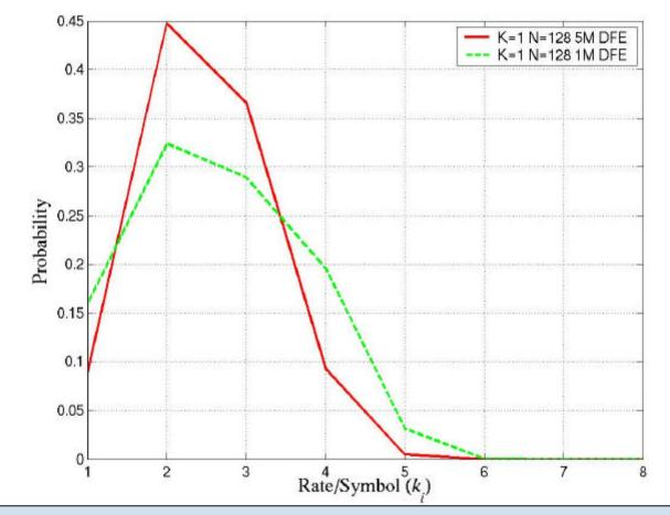
Probability of using rate  $k_i$  in a single user case with both 1 Mhz and 5 MHz bandwidth
