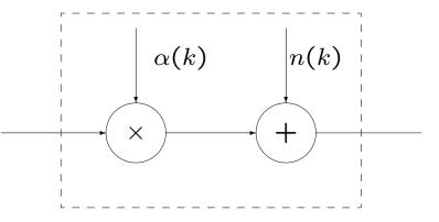
Introduce  $\gamma = \bar{P}\alpha/N_0B$ , where  $\bar{P}$  is the average power into the channel Let the instantaneous power vary  $\rightarrow$  Instantaneous CSNR:  $\gamma P/\bar{P}$ Channel capacity per channel use for this CSNR:
