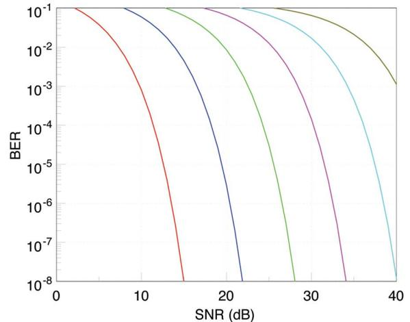
**Fig. 1. BER versus SNR per symbol for Gray coded QAMs. The curves from left to right correspond to 2, 4, 6, 8, 10, and 12 bits per symbol.**
