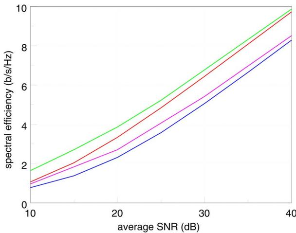
**Fig. 7. Maximum spectral efficiency versus SNR per symbol for adaptive QAM modulations with adaptive power only when  $N = 6$  and  $BER_{dg} = 0.001$  (green) and  $N = 6$  and  $BER_{dg} = 10^{-7}$  (magenta). These schemes are designed to have  $BER = BER_{dg}$  for all SNRs. The corresponding curves for an adaptive rate only scheme, designed to have  $BER \leq BER_{dg}$ , (from Fig. 5) are also shown (red and blue).**
