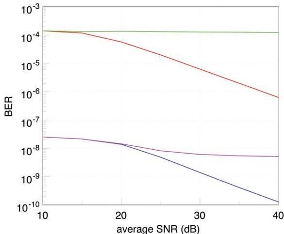
**Fig. 6.** Average BER versus SNR per symbol for adaptive QAM modulations with adaptive rate only when  $N = 3$  and  $BER_{dg} = 0.001$  (red),  $N = 3$  and  $BER_{dg} = 10^{-7}$  (blue),  $N = 6$  and  $BER_{dg} = 0.001$  (green), and  $N = 6$  and  $BER_{dg} = 10^{-7}$  (magenta). These schemes are designed to have  $BER \leq BER_{dg}$ .
