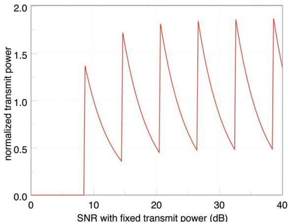
**Fig. 10.**  $S(\gamma)/\bar{S}$  for the adaptive power and rate scheme designed for an instantaneous BER of 0.001 when the average SNR ( $\bar{\Gamma}$ ) is 30 dB. Please refer to the legend of Fig. 8 for further explanation of the curve.
