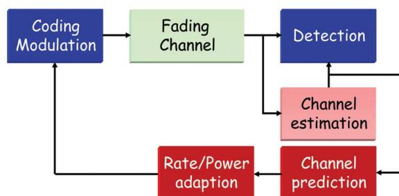
**Fig. 4.** Major functions in an adaptive modulation system.
