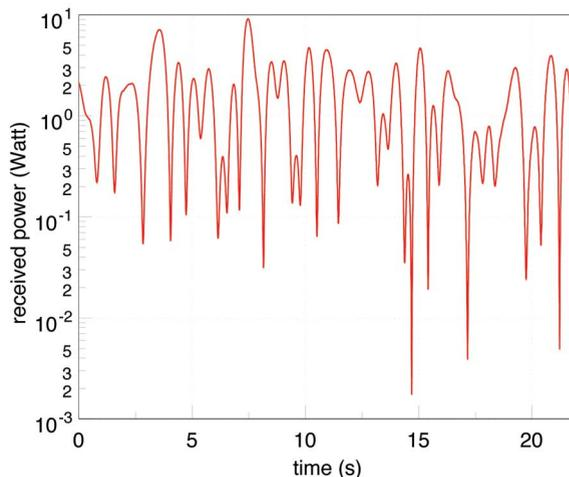
**Fig. 2.** Example of received power versus time when a sinusoidal tone with constant power is transmitted on a flat Rayleigh-fading channel. The Doppler frequency is 1 Hz. The time axis will scale with the inverse of the Doppler frequency for other Doppler frequencies.
