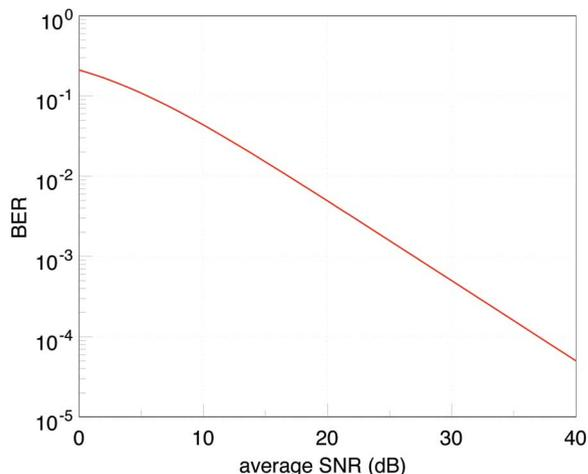
**Fig. 3.** BER versus SNR per symbol for QAMs with 2 bits per symbol on a Rayleigh-fading channel.
