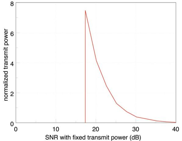
**Fig. 8.  $S(\gamma)/\bar{S}$  for the adaptive power and constant rate scheme, designed for  $BER = BER_{dg} = 0.001$ , when the average SNR ( $\Gamma$ ) is 30 dB. The SNR on the abscissa is the SNR in the receiver when a fixed power equal to  $\bar{S}$  is transmitted. This SNR is directly related to the channel power gain. The actual SNR in the receiver is equal to the product of the corresponding values on the horizontal axis and vertical axis.**
