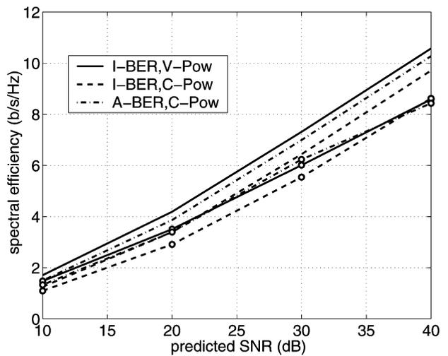
**Fig. 13.** Maximum spectral efficiency versus SNR per symbol for adaptive QAM modulations which are optimized for predicted channel power gains. The design BER is 0.001. The lines without a marker are for  $\sigma_{\epsilon_p}^2 = 0.001$  and the lines with the rings are for  $\sigma_{\epsilon_p}^2 = 0.1$ . (From [2], copyright IEEE 2004.)
