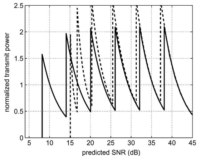
**Fig. 11.**  $S(\hat{\gamma})/\bar{S}$  for the adaptive power and rate scheme designed for an instantaneous BER of 0.001 when the average SNR ( $\Gamma$ ) is 20 dB. Solid and dashed lines correspond to  $\sigma_{\epsilon_p}^2 = 0.001$  and  $\sigma_{\epsilon_p}^2 = 0.1$ , respectively. (From [2], copyright IEEE 2004.)
