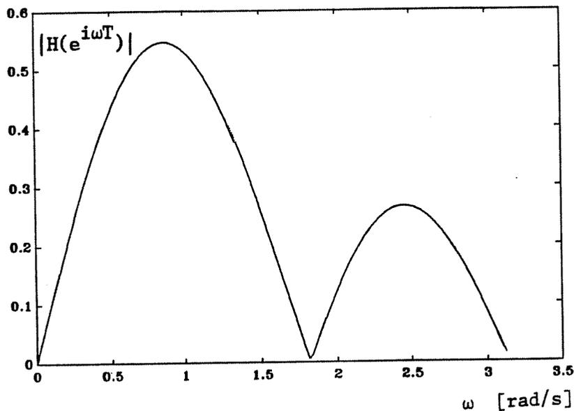
Figure 4.2. Amplitude response of a second order least squares polynomial differentiator based on 5 data points, ( $T=1$ ).
