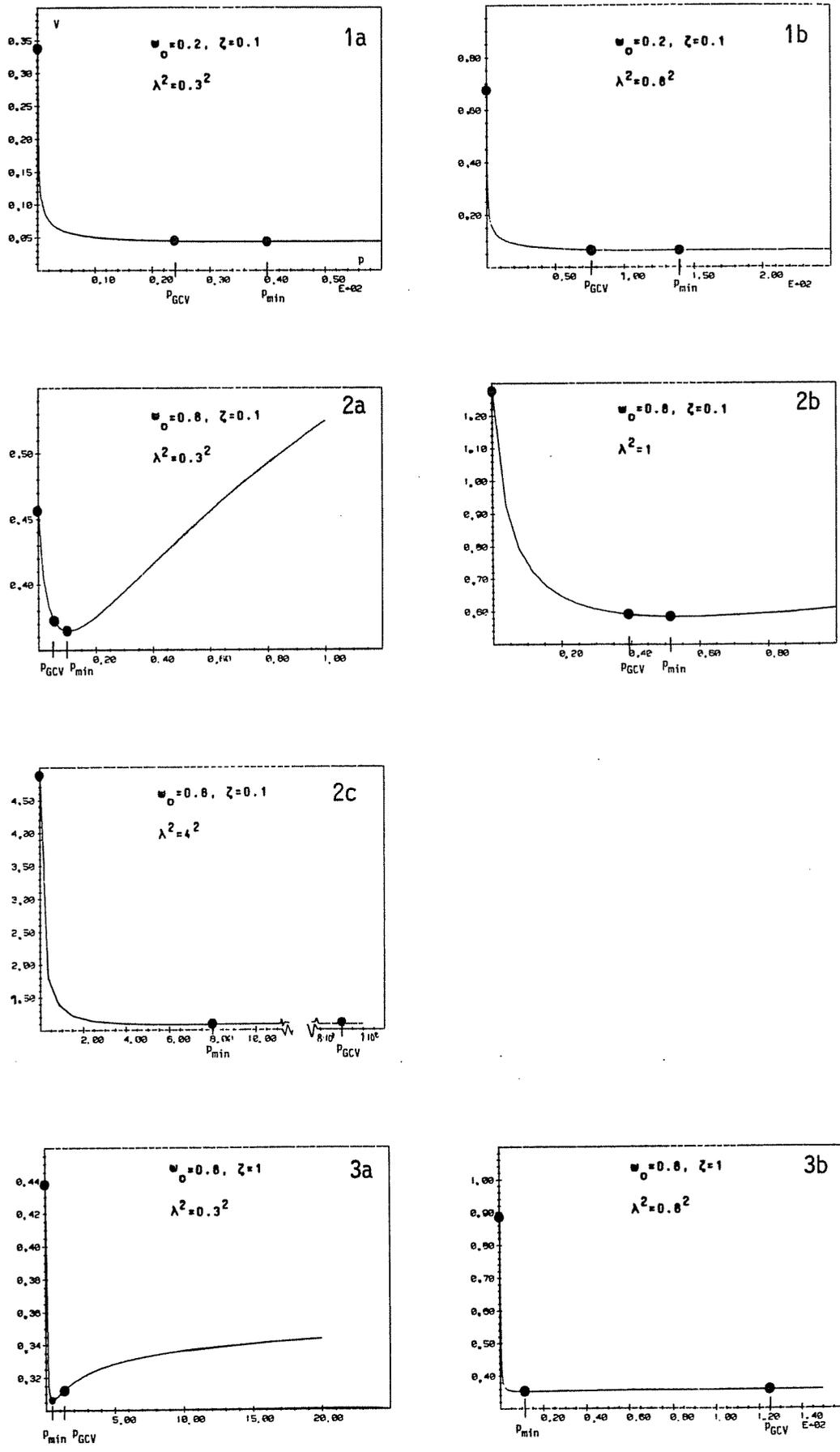
**Figure 5.3.** The loss function  $V$  as a function of the regularizing parameter  $p$  for  $m=2$  (i.e. cubic regularized splines).
