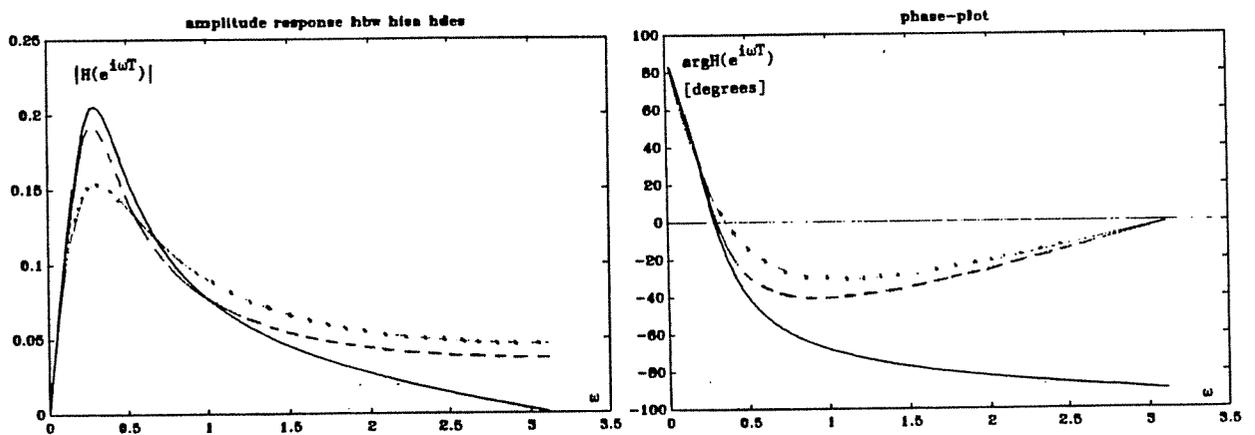
Figure 5.10. Magnitude and phase of the frequency responses,  $H_{BW}$  (---),  $H_{IEA}$  (-·-·-),  $H_{DES}$  (····).
