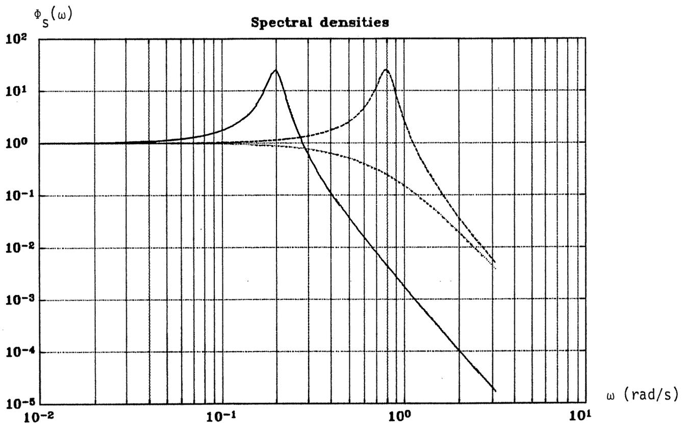
Figure 5.1. Spectral densities for the signals,  $\omega_0=0.2$ ,  $\zeta=0.1$  (—),  $\omega_0=0.8$ ,  $\zeta=0.1$  (---),  $\omega_0=0.8$ ,  $\zeta=1$  (···).
