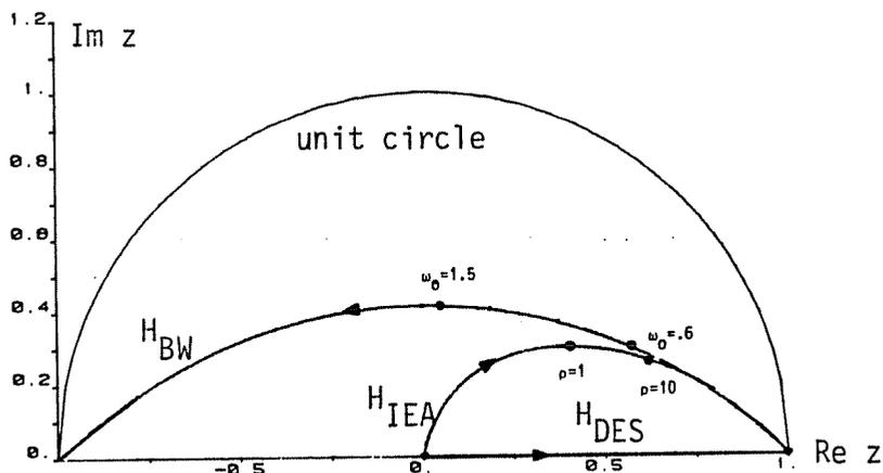
**Figure 5.9.** Poles of the filters as a function of the design parameters.
