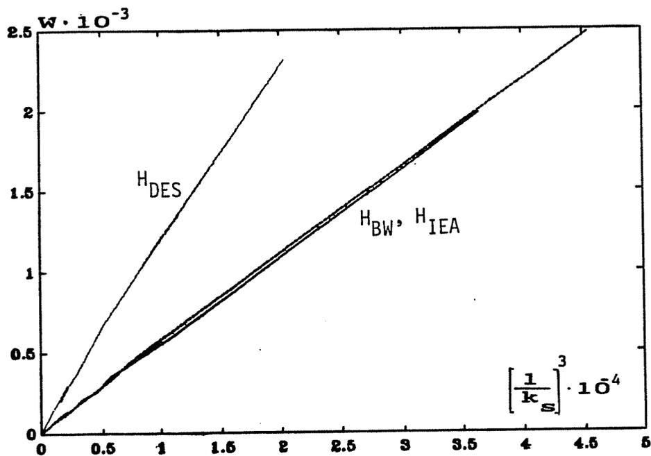
Figure 5.7a. Noise transmission as a function of the cubed inverted settling time.
