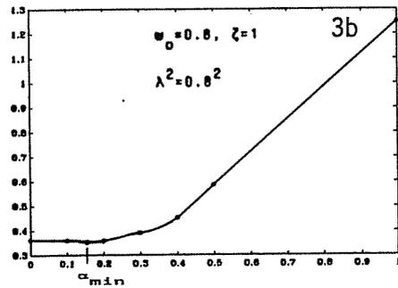
Figure 5.4. The loss function  $V$  as a function of the parameter  $\alpha$ .
