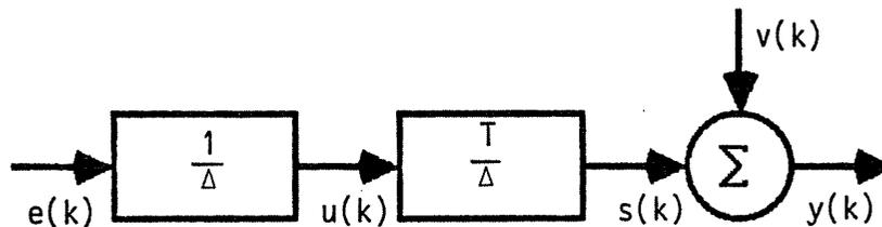
Figure 5.6. A discrete-time input estimation approach for tracking the derivative of a noisy trend signal with abrupt changes in the derivative.
