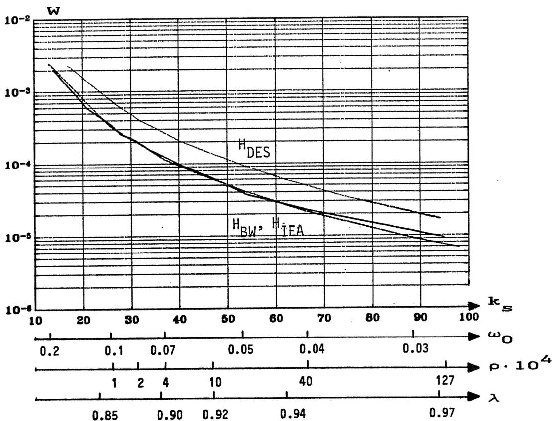
Figure 5.7b. Noise transmission as a function of the settling time and the filters design parameters.
