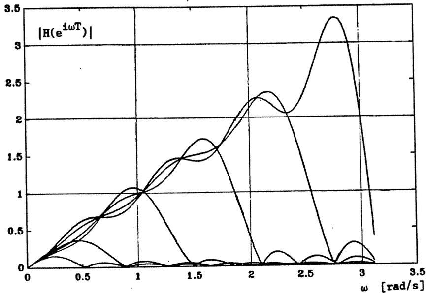
Figure 5.5. Amplitude responses for the UA-method,  $\alpha=0, 0.2, 0.4, 0.6, 0.8, 1$ .
