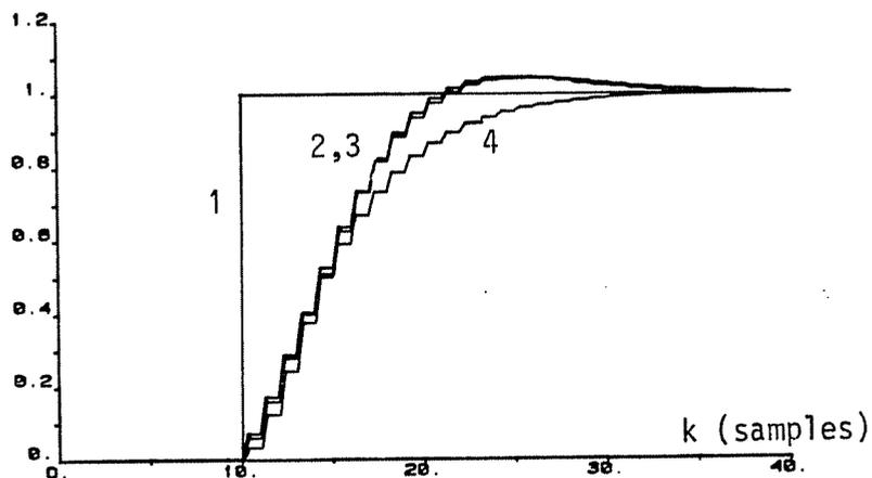
Figure 5.8. Step responses for the filters. The true derivative (1), the filter  $H_{BW}$  (2),  $H_{IEA}$  (3) and  $H_{DES}$  (4).
