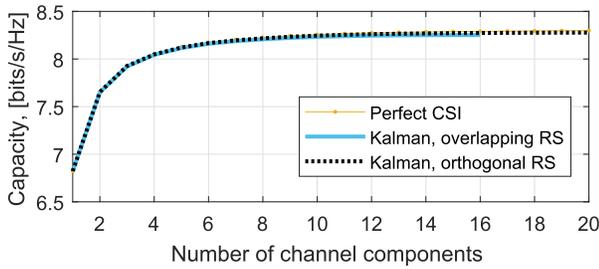
Fig. 5. An illustration of the single users maximum ratio beamforming gain, based on Shannon capacity, as a function of the included number of channel components. CSI accuracy is based on the Kalman estimates in Figure 4a. Note that the curves overlap.
