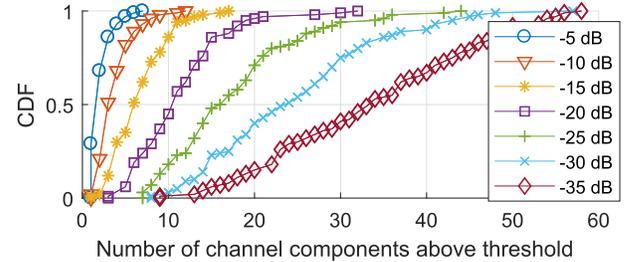
Fig. 3. CDF of the number of relevant channel components (CCs) at different user positions when using different thresholds (in dB) relative to the power of the strongest channel.
