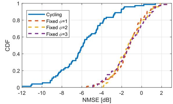
Fig. 6. Comparison of the NMSE distributions of channel estimates based on cycling and non-cycling (fixed) RSs, as in Figure 2. The statistics represent the 72 i.i.d. channels.
