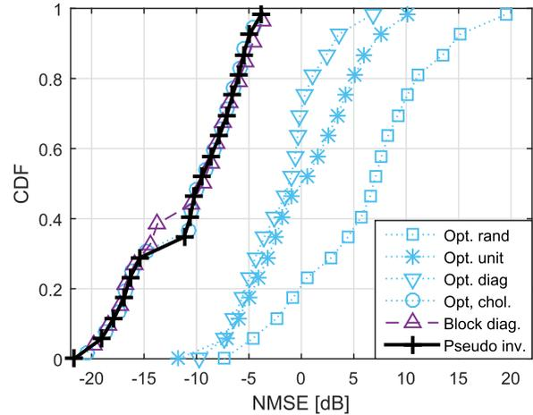
Fig. 7. The CDFs of the NMSE provided by the reduced Kalman filter using estimates of the process noise matrix  $Q$  through (17), denoted “Pseudo inv.”, through optimization of an upper triangular matrix  $M$  in (18), denoted “Opt.”, with different initial values for  $M$ , and by using a block diagonal channel covariance matrix  $R_h$  to find a block diagonal  $Q$  through (16), denoted “Block diag.”.
