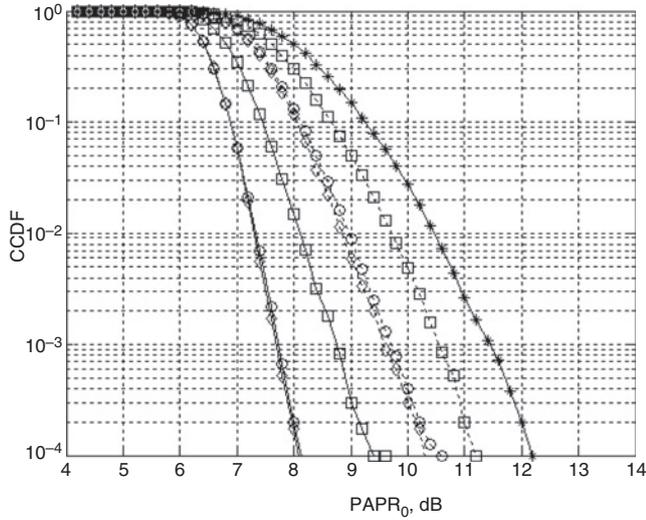
**Fig. 1** CCDFs of AP-PTS, existing IP-PTS and EIP-PTS
