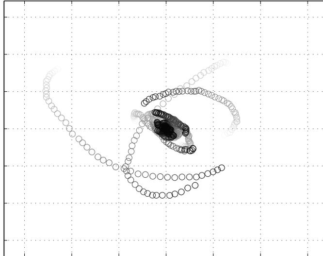
Figure 3.3: Impulse response measurements of a 1800 MHz radio channel in suburban Stockholm. The received signal was correlated with the known transmitted sequence. The figure has no particular scaling, but both axes span the same range.
