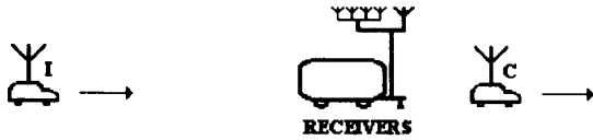
Fig. 7: The figure shows how the mobile transmitting the interfering signal was placed 180 degrees from the beam maximum. C was moving away from the receivers. I was moving towards them or not moving at all (different tests).
