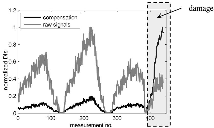
Figure 5. Comparison of damage indices calculated using cross correlation between the raw and the temperature-compensated signals. The measurements with gray background were taken for the damaged plate.
