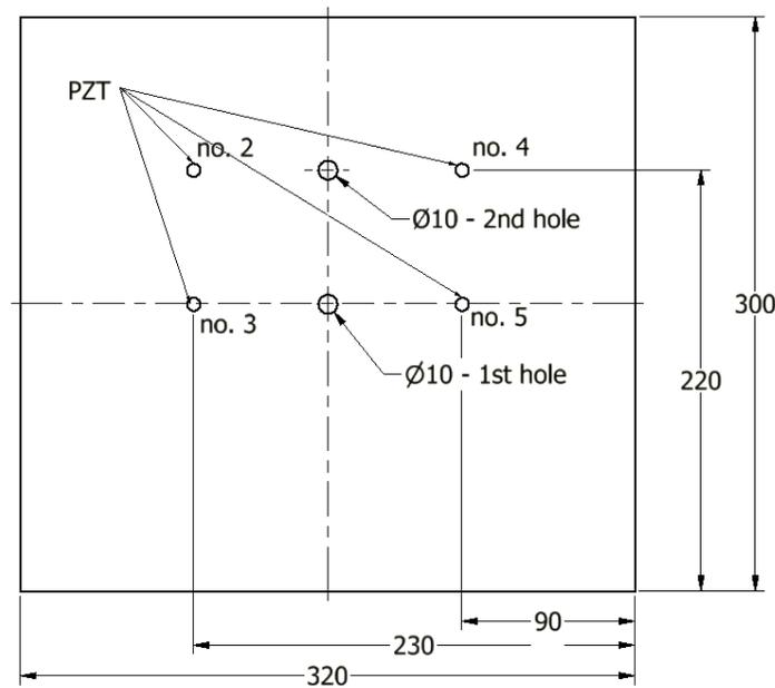
Figure 1. The specimen used in the experiment
