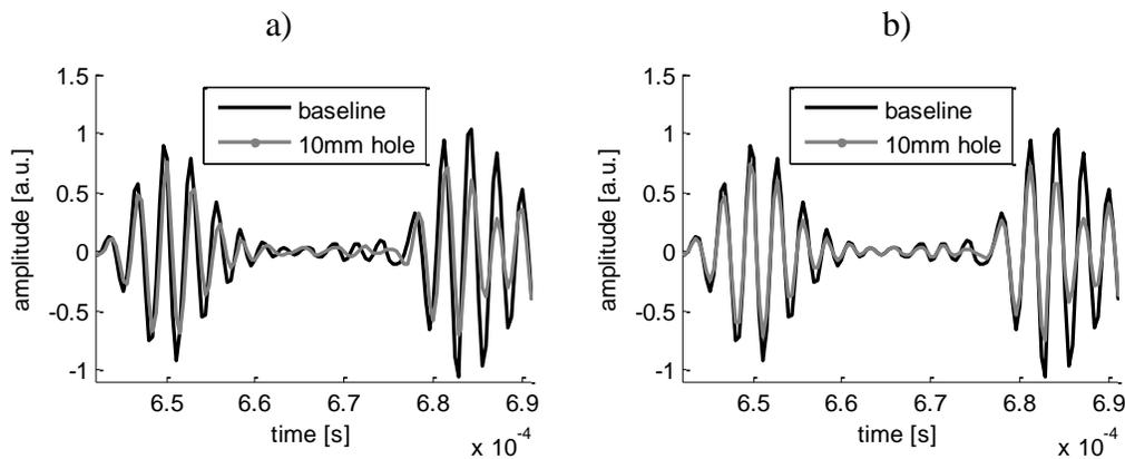
Figure 4 a) Comparison of baseline and damaged signals acquired at room temperatures b) result of the compensation procedure applied to the damaged signal.
