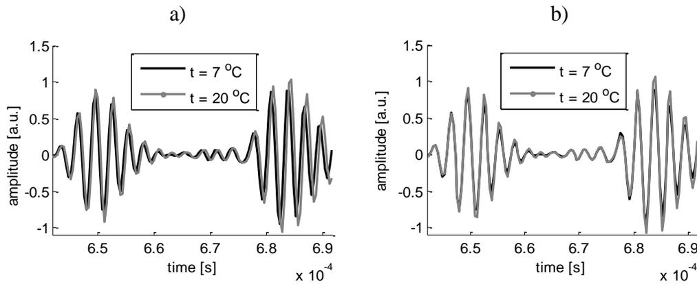
Figure 3. Example of time signals acquired for an intact plate a) affected by temperature change b) after compensation.
