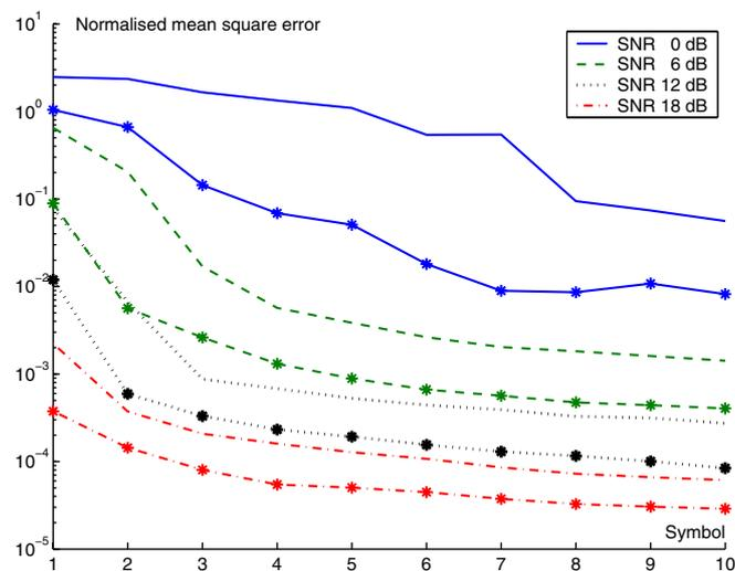
Figure 1. The performance of the ignorant receiver can improve quite significantly when consecutive symbols are used. Two extra symbols can give an improvement of up to 100 times at an SNR of 12 dB, no oversampling (—). Oversampling of the signal (—\*) yields a noticeable error reduction.
