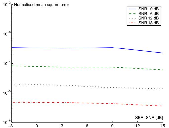
Figure 5. Nulling of subcarriers in an OFDM pilot seems to render the channel predictions almost useless for the well-informed receiver, unless they are of extremely good quality. This also means that the ignorant receiver, if it knew the locations of the nulls, could perform very well with sparse pilots.
