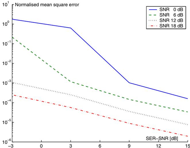
Figure 4. Access to pilots and channel predictions can substantially increase the estimation accuracy. This fact can be exploited when fine-tuning the local oscillator during operation.
