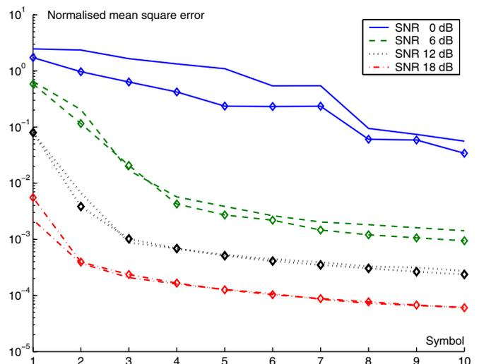
Figure 3. Simulations support the use of the variance of the posterior (—◇—) as an indicator of when the mobile is sufficiently synchronised to the system. It is here compared with the actual error in the simulations (—).
