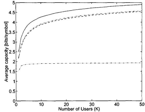
Fig. 5. Spectral efficiency (23) when all users have average SINR 16 dB, and the user with highest SINR among  $K$  terminals with Rayleigh fading channels is selected. Solid: perfect prediction. Dash-dotted: prediction NMSE  $\sigma^2_{\Delta\gamma/\gamma} = 0.1$ , with optimized rate limits. Dashed: prediction NMSE 0.1, rate limits as for perfect prediction. Lower dash-dotted: NMSE 0.495.
