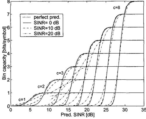
Fig. 1. Bin capacity  $b_{u,\ell}$  by (17) as a function of the instantaneous SINR for SINR prediction NMSE 0.1 and  $n_s = 108$ , at modulation rates  $c_{u,\ell} \in [1, \dots, 8]$ , for average SINR 0 dB (solid), 10 dB (dashed) and 20 dB (dash-dotted). Compare to perfect prediction (dotted).
