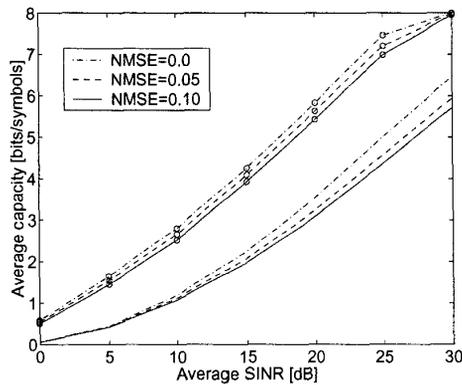
Fig. 3. Spectral efficiency (23) as a function of the average SINR which is equal for all users, for  $K = 1$  terminal (lower curves) and  $K = 20$  (upper curves with markers). Results for perfect predictions (dash-dotted) NMSE 0.05 (dashed) and NMSE 0.10 (solid).
