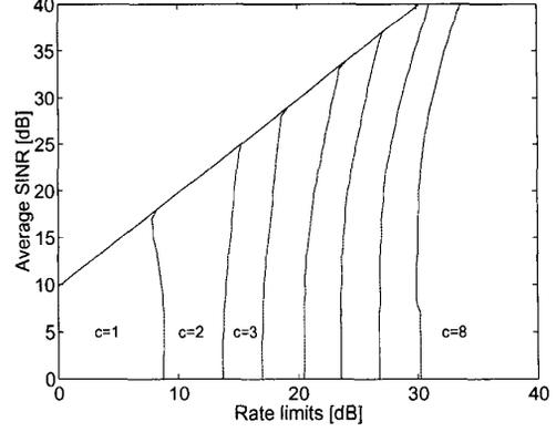
Fig. 2. Optimized modulation rate limits for modulation rates  $c_{u,\ell} \in [1, \dots, 8]$  as a function of the average SINR when the SINR prediction NMSE is 0.1. The diagonal line represents the lower limit  $\hat{\gamma}/\bar{\gamma} \geq \bar{\sigma}^2$  for predicted SINR's obtained by the unbiased predictor.
