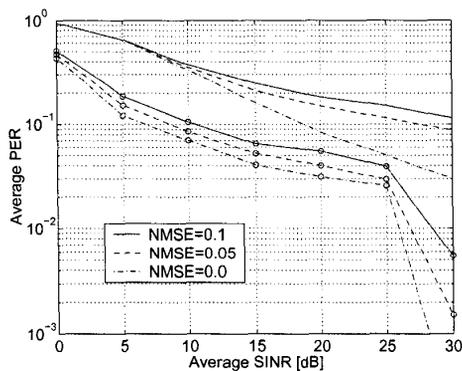
Fig. 4. Average frame error rate as a function of the average SINR, which is equal for all users, for  $K = 1$  and  $K = 20$  terminals (with markers). Results for 108 symbols per frame.
