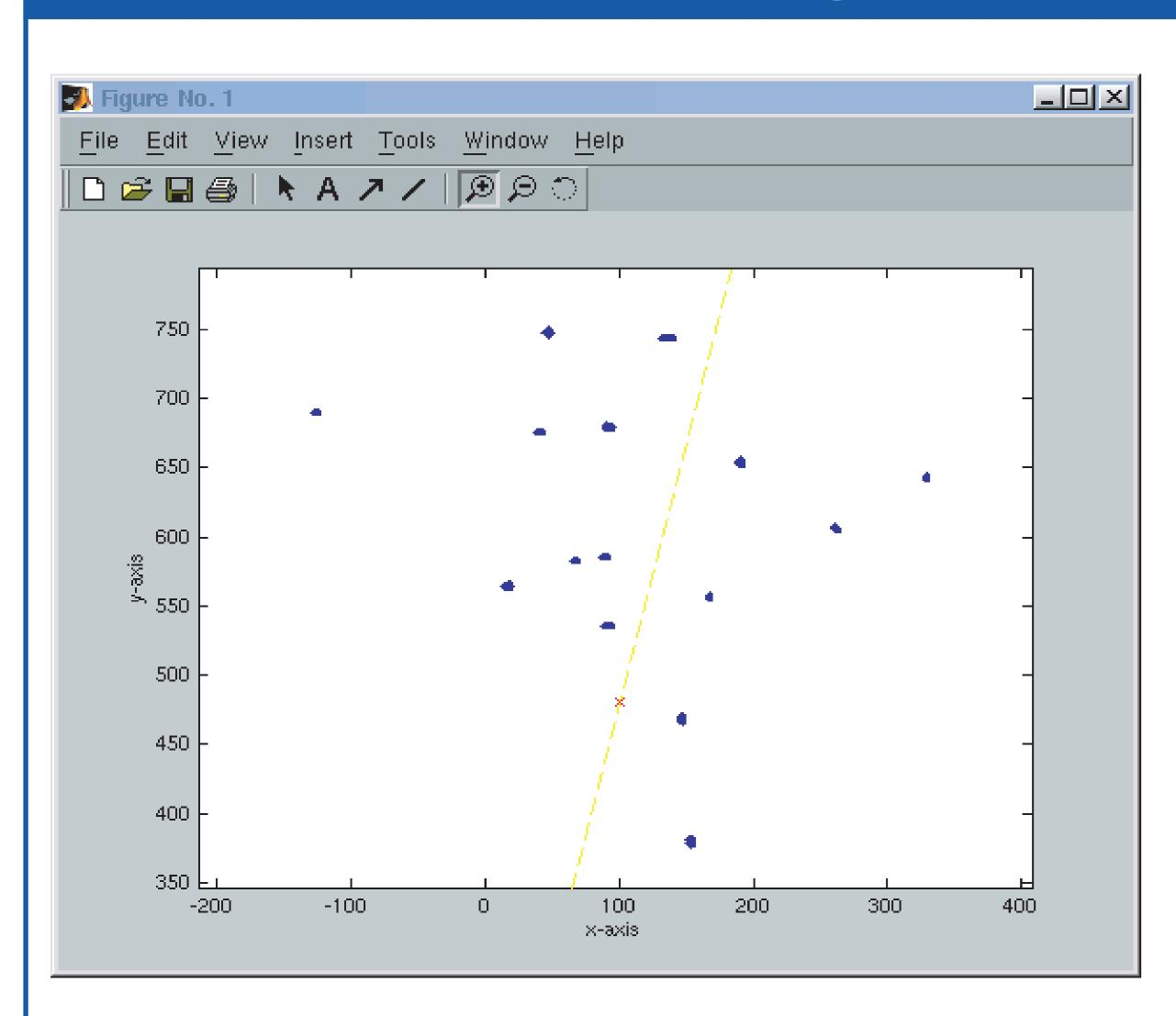
The mobile moves at constant speed along the yellow path. It is surrounded by radio wave scattering objects that create multipath propagation of the received
