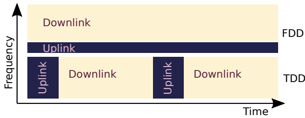
Figure 1.3. Uplink and downlink resource allocation for FDD and TDD systems respectively.
