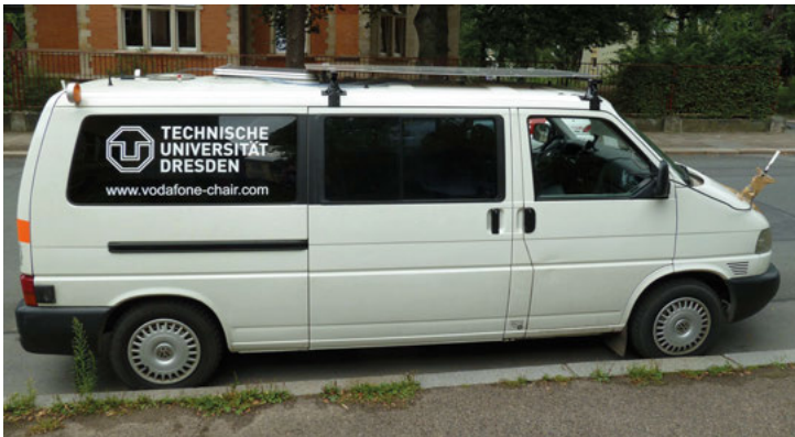
Figure 4.19. Measurement set-up for the measurements collected in downtown Dresden. The metal sheet with the four antennas was placed on top of a measurement van.
