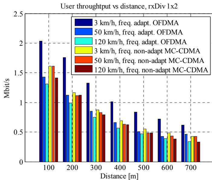
**Figure A-9: Receive diversity 1x2 scheme for frequency adaptive (SB) and non-adaptive (RR) allocation: user throughput as a function of the distance.**
