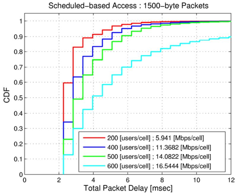
Figure A-24: 1500-byte Packets without DAC
