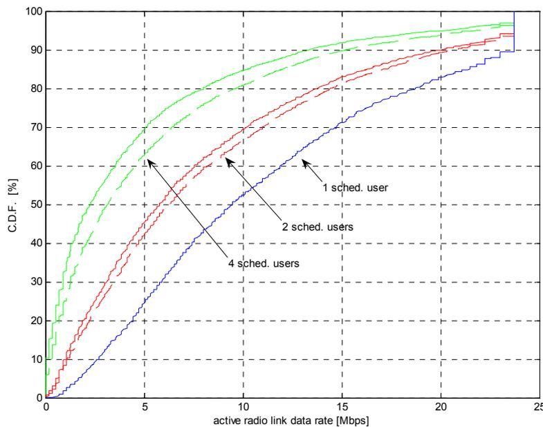
**Figure A-29: Distribution of the active radio link data rates with 1, 2, and 4 SDMA users without (-) and with (- -) SIC. Power control is not used.**
