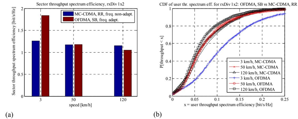
**Figure A-8: Receive diversity 1x2 scheme for frequency adaptive and non-adaptive allocation: sector throughput spectrum efficiency [bit/s/Hz] for as a function of UT speed (a); cumulative distribution function of user throughput efficiency (b).**
