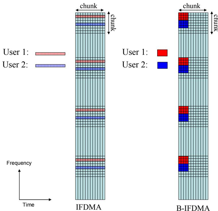
**Figure B-10: Example of B-IFDMA based on current FDD chunk size. Note that the appropriate block size is to be determined.**
