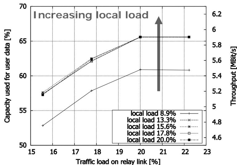
Figure C-18: Throughput with FDT - rising load on relay connection
