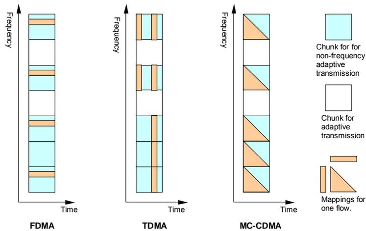
**Figure B-1: Illustration of the different flow mapping strategies onto chunks as considered in WINNER I [WIND210].**
