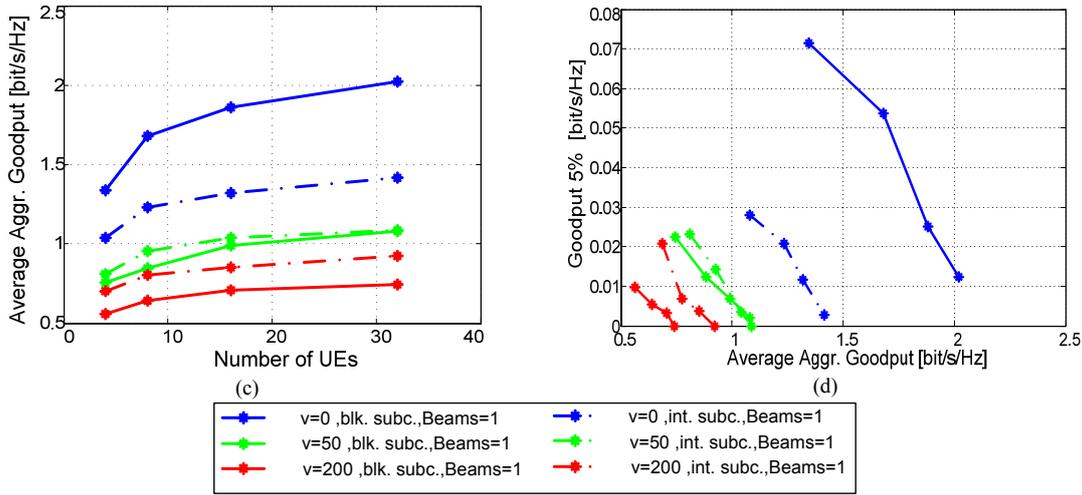
**Figure A-3: Average aggregate system goodput comparison for adaptive (chunk) and non-adaptive (interleaved) frequency allocation at different terminal velocities, CSI update (a, b) rate 1 and (c,d) rate 8.**
