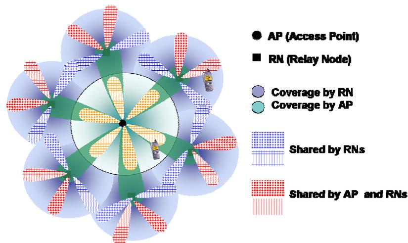
**Figure 4-3:** Example of beam pattern configuration for the RNs of one REC (AP means BS in the figure).
