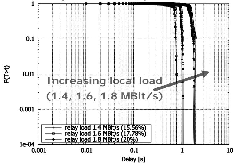
Figure C-16: Downlink end-to-end delay without FDT
