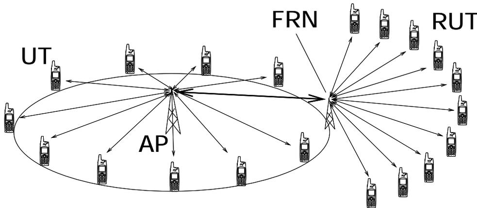
Figure C-5: Frame-by-frame multi-hop scenario
