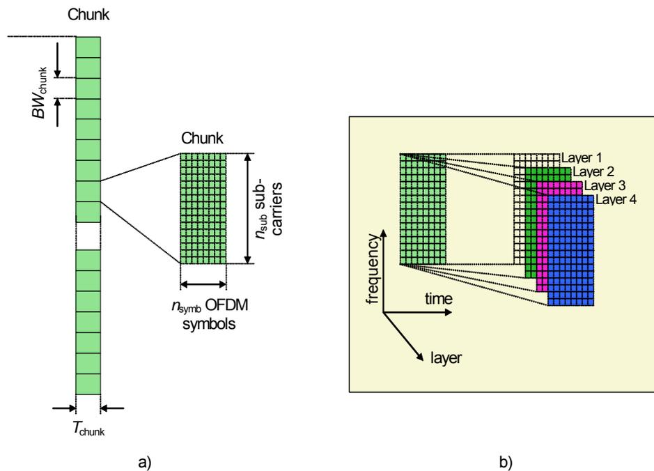
**Figure 1-1: a) Multi-carrier Downlink physical channel structure and chunks. b) Chunk layers obtained by spatial re-use.**
