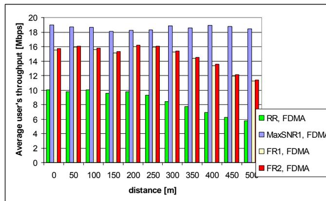
**Figure A-12 Average user's throughput vs. distance between BS and UT**
