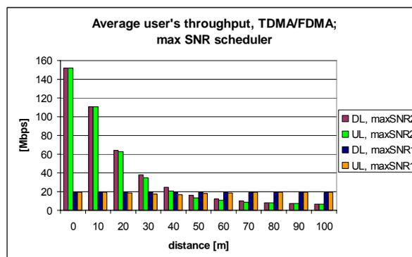
**Figure A-17. Average user’s throughput vs. distance for the MaxSNR schedulers, 40 users allocated**
