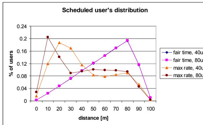
**Figure A-16. Distribution of scheduled users vs. distance for two types of user’s scheduling: fair time sharing and maximum rate sharing; 40 and 80 users allocated**
