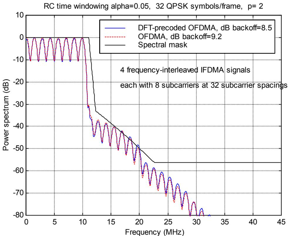
**Figure B-9: HPA output power spectra for OFDMA and for 4 frequency-interleaved IFDMA signals with 10 MHz nominal bandwidth. HPA has Rapp model nonlinearity with parameter  $p=2$ .**
