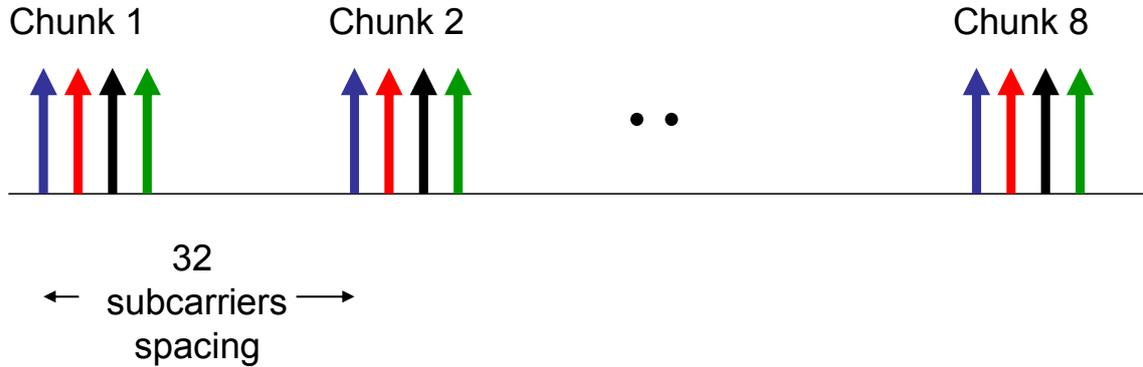
**Figure B-8: Frequency domain illustration of a signal with 128 subcarriers, consisting of 4 frequency-interleaved IFDMA signals, each with 8 subcarriers, and with subcarriers at 32-subcarrier intervals.**
