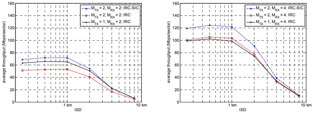
**Figure A-35: Average downlink sector throughput with two (left) and four (right) terminal receive antennas as a function of the site-to-site distance.**
