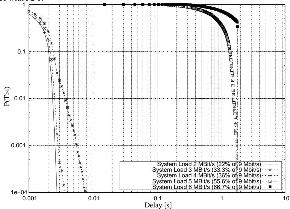
Figure C-9: Pdf of downlink delay vs Load using Round Robin scheduling without FDT
