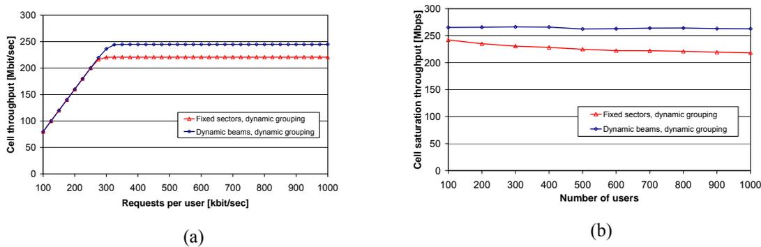
**Figure A-11: Cell throughput achievable through dynamic spatial resource sharing in RECs.**
