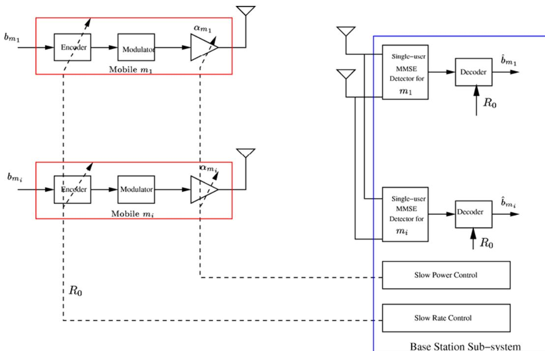
Figure 3-2: Terminal transmitters and a base station receiver.
