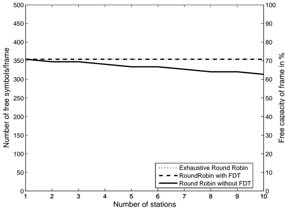
**Figure C-7: Comparison of free symbols in a MAC frame in the case of multi-hop**
