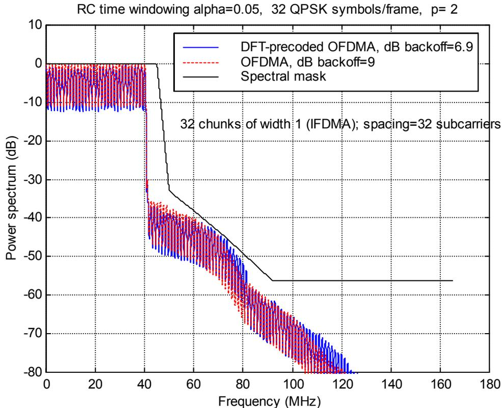
**Figure B-4: HPA output power spectra for OFDMA and DFT-precoded OFDMA signals corresponding to IFDMA with 40 MHz nominal bandwidth. HPA has Rapp model nonlinearity with parameter  $\rho=2$ .**
