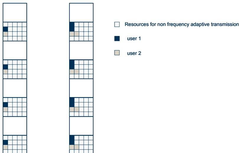
**Figure 3-1: Two example of resource usage for non-frequency adaptive uplink transmissions. Time is in the horizontal direction, frequency in the vertical. The large dotted areas are chunks and the small squares represent blocks. Pilots for channel estimation are included in each block.**
