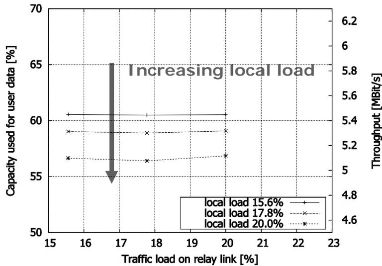
Figure C-15: Throughput without FDT - rising load on relay connection
