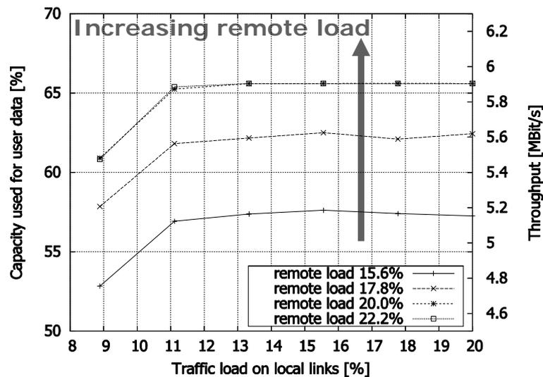
Figure C-17: Throughput with FDT - rising load on local connections
