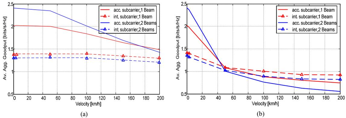
**Figure A-4: Average aggregate system goodput vs. terminal velocity for adaptive and non-adaptive frequency allocation, CSI update (a) rate 1 and (b) rate 8.**
