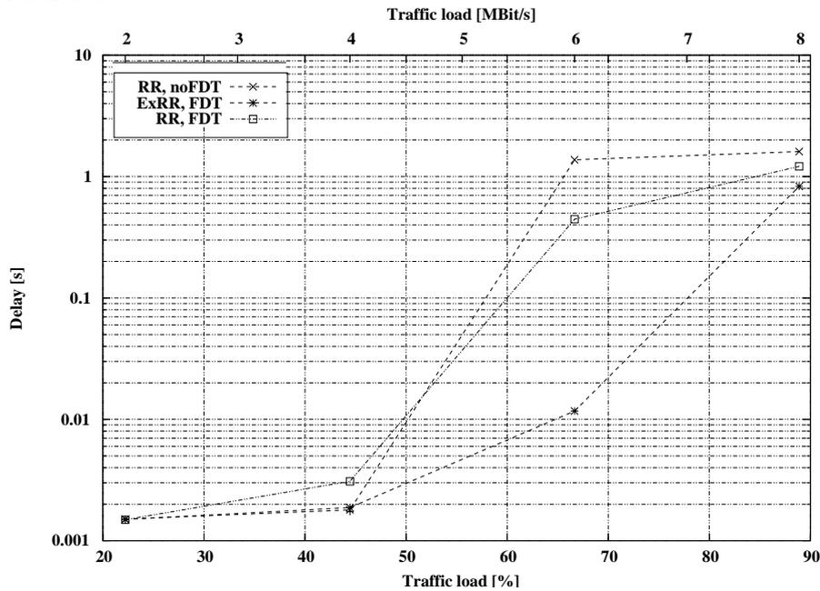
Figure C-13: Mean downlink delay vs. System Load depending on scheduling algorithm
