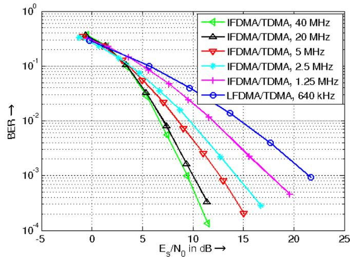
**Figure A-23. Performance results for SISO transmission of IFDMA/TDMA for different bandwidths and for LFDMA/TDMA as reference, 16 subcarriers per user**
