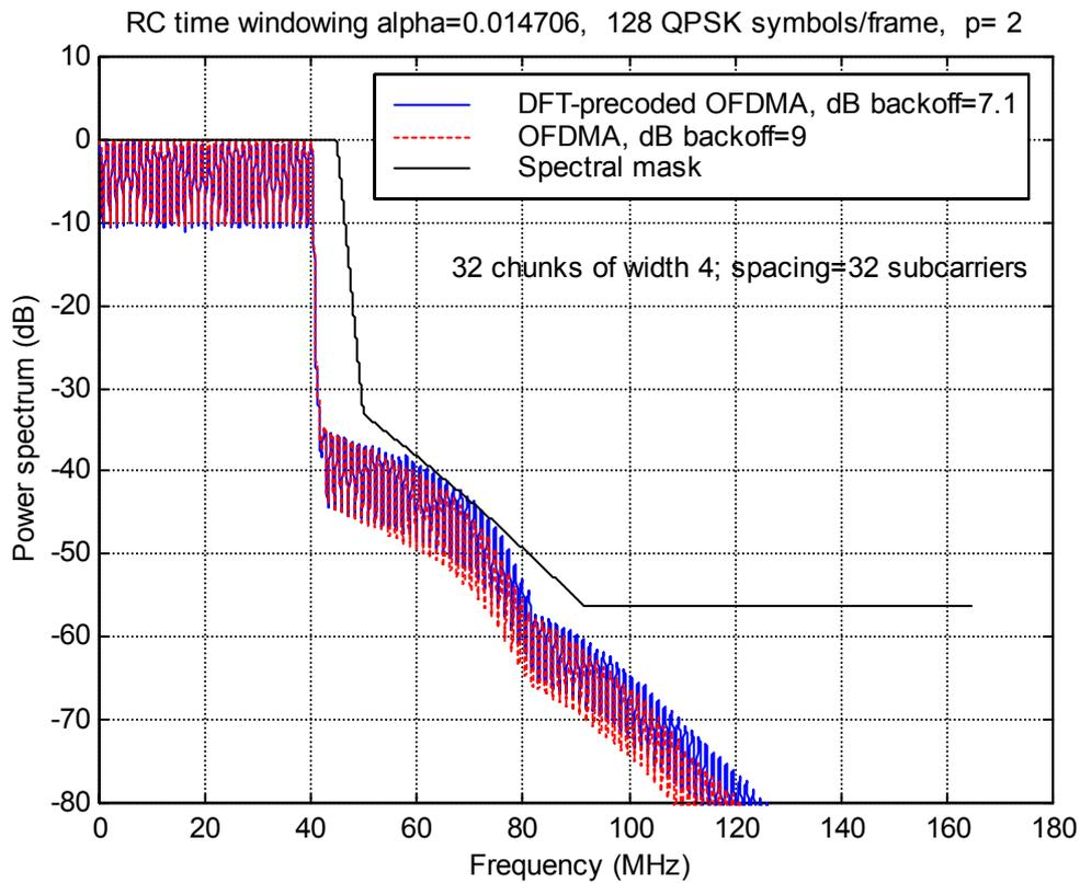
**Figure B-5:** HPA output power spectra for OFDMA and DFT-precoded OFDMA signals with chunk width=4 and with 40 MHz nominal bandwidth. HPA has Rapp model nonlinearity with parameter  $p=2$ .
