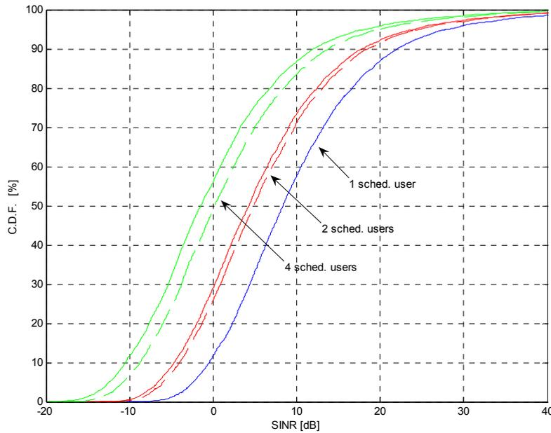
**Figure A-28: Post-receiver SINR for 1, 2, and 4 scheduled users. Power control is not used. Performance without (-) and with (- -) SIC is depicted.**
