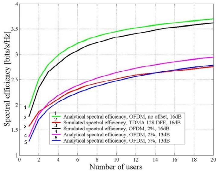
**Figure A-31: Performance of the Adaptive Uplink under different frequency offsets as a fraction of the subcarrier spacing. As a comparison, the results of the adaptive TDMA uplink presented in [WIND210] section G4.1 is also shown.**
