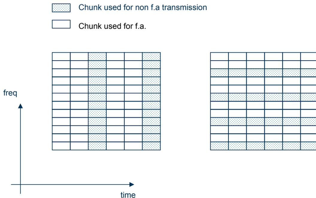
**Figure 5-1: Time and frequency multiplexing of resources used for frequency adaptive and non-frequency adaptive transmission.**
