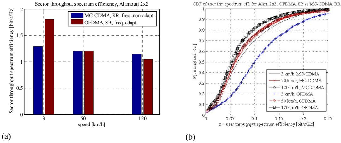
**Figure A-7: MIMO Alamouti 2x2 scheme for frequency adaptive and non-adaptive allocation: sector throughput spectrum efficiency [bit/s/Hz] for as a function of UT speed (a); cumulative distribution function of user throughput efficiency (b).**
