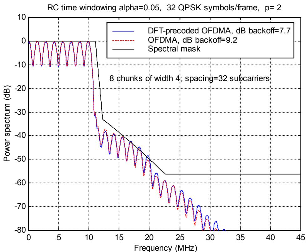
Figure B-7: HPA output power spectra for OFDMA and DFT-precoded OFDMA signals with chunk width=4 and with 10 MHz nominal bandwidth. HPA has Rapp model nonlinearity with parameter  $p=2$ .
