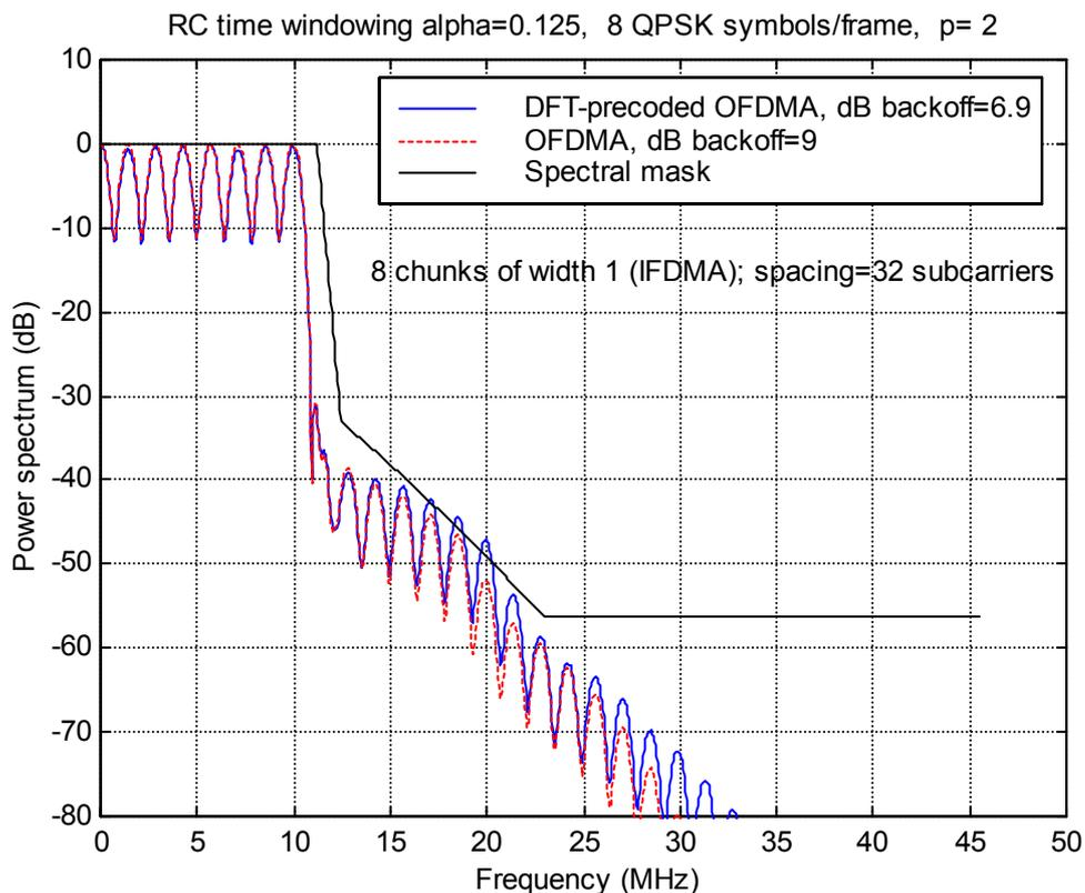
Figure B-6: HPA output power spectra for OFDMA and DFT-precoded OFDMA signals corresponding to IFDMA with 10 MHz nominal bandwidth. HPA has Rapp model nonlinearity with parameter  $p=2$ .
