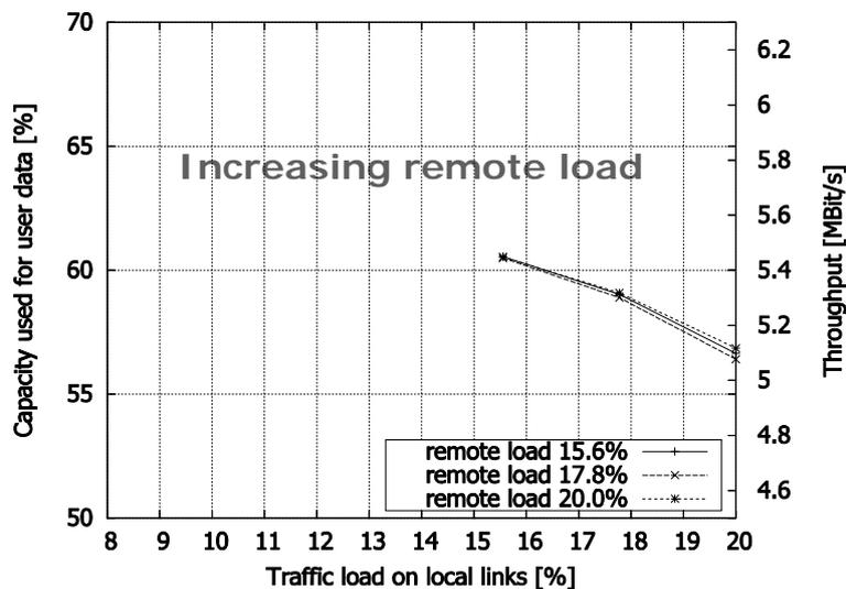
**Figure C-14: Throughput without FDT - rising load on local connections**
