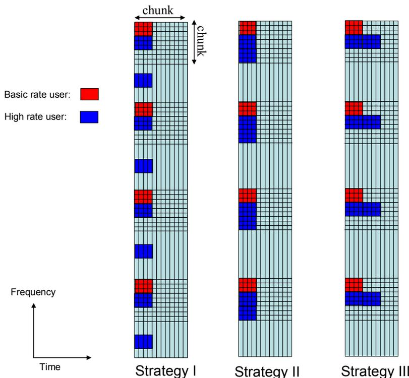
**Figure B-11: Illustration of flexible resource allocation in B-IFDMA and B-EFDMA. Note that the appropriate block size is to be determined.**
