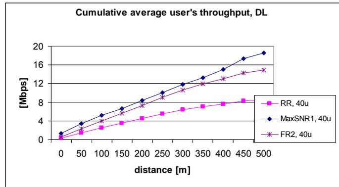
**Figure A-13. Cumulative distribution of average user’s average throughput normalized to the scheduled user’s spatial density for TDMA/FDMA shown as a function of distance**
