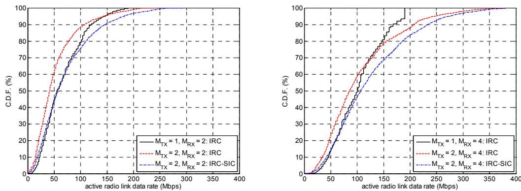
**Figure A-34: Active radio link data rate distributions with two (left) and four (right) terminal receive antennas, respectively.**
