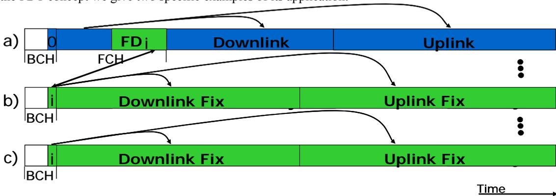
**Figure C-2: FD describing a Static Frame**
