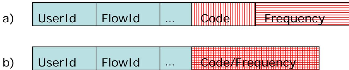
**Figure 7-2: Adaptable control information structure**
