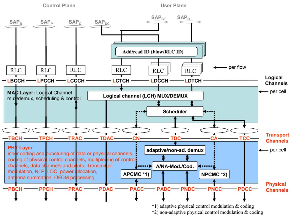
Figure 7-1: Radio Interface Protocol architecture (network side)
