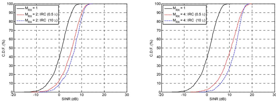
**Figure A-36: Post receiver SINR in a multi-cell deployment with different number of base station antennas (1, 2, and 4) and different antenna separations (0.5 and 10 wavelengths). IRC is used and the inter-site distance is 250 m.**
