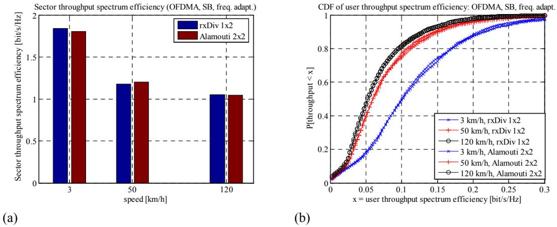
**Figure A-5: Adaptive frequency allocation, OFDMA/TDMA, Score Based scheduling: sector throughput spectrum efficiency [bit/s/Hz] for as a function of UT speed (a); cumulative distribution function of user throughput efficiency (b).**
