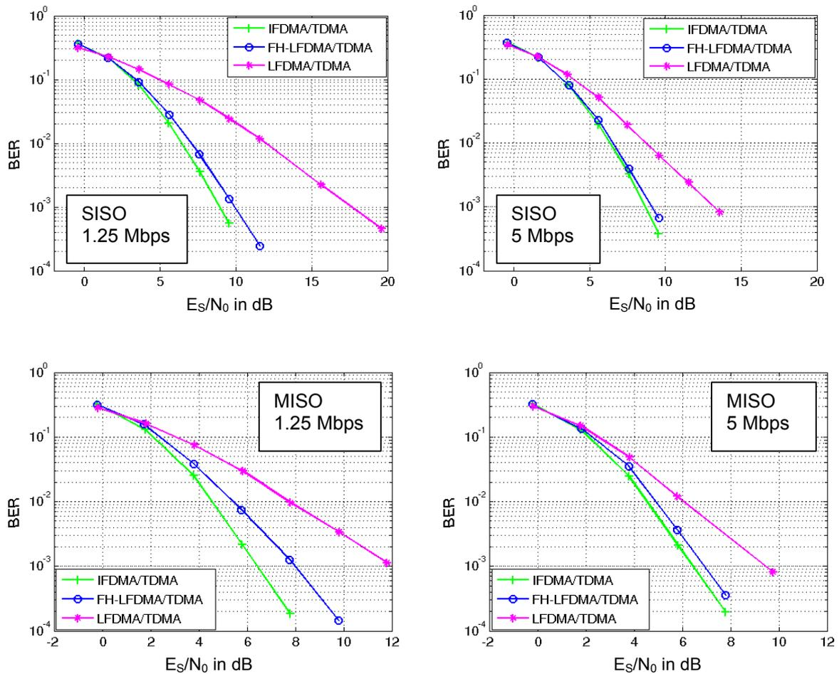
Figure A-22. Performance results for SISO and MISO transmission of LFDMA/TDMA, FH-LFDMA/TDMA and IFDMA/TDMA in a Wide Area scenario for different data rates
