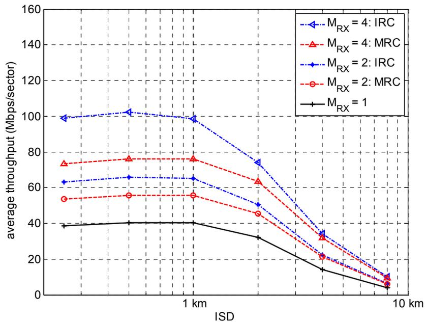
**Figure A-33: Downlink average sector throughput as a function of the inter-site distance for different number of receive antennas (1, 2, and 4) and for different combining schemes (MRC and IRC).**
