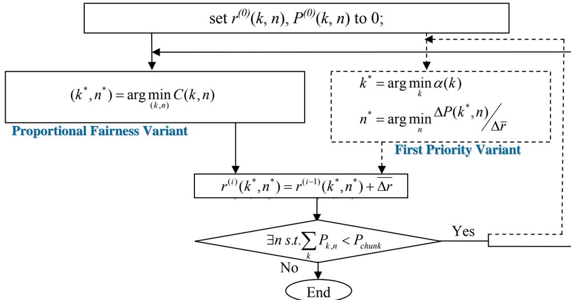
Figure 4-2: Greedy algorithm for joint FDMA/SDMA resource allocation
