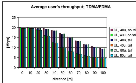
**Figure A-15. Average user's throughput vs. distance for cells with 40 and 80 users; coding with and without tail, Round Robin scheduling**
