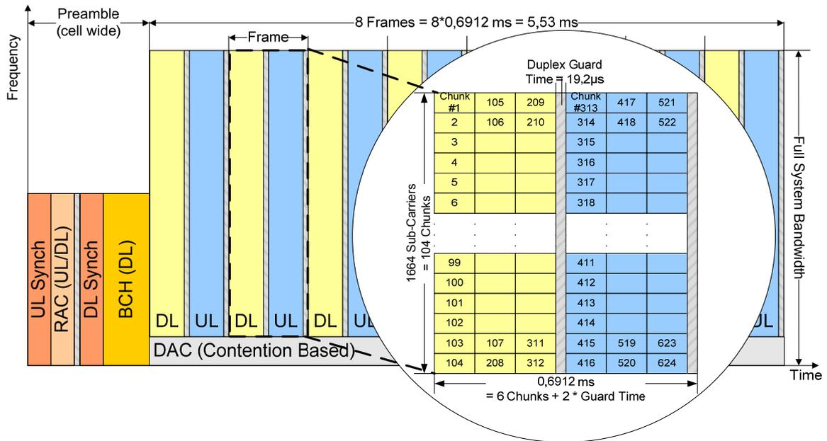
Figure 1-2: Superframe example (from [WIND210], numbers are subject to change) with eight TDD frames and asymmetry 1:1, a preamble containing a broadcast channel (BCH) and synchronization pilots, and a set of frequencies reserved for contention based peer-to-peer communication. The frame for TDD cellular transmission with its chunk-based substructure (from [WIND210], numbers are subject to change) has been enlarged.
