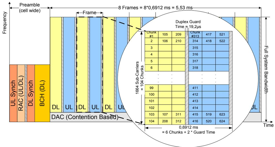
**Figure A-2: Sketch of superframe structure (holds for both FDD and TDD scenarios) and frame structure (holds only for microcellular and indoor test scenarios).**
