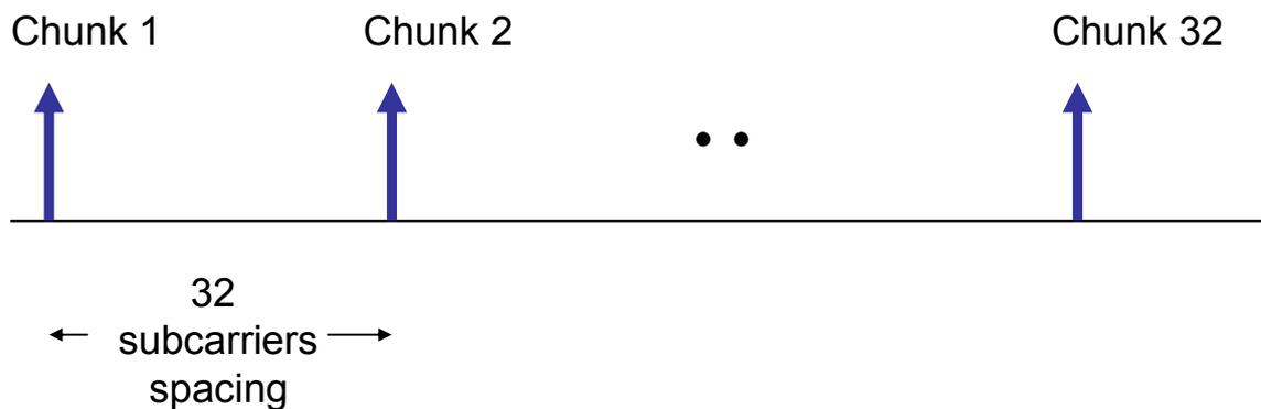
**Figure B-2: Frequency domain illustration of an IFDMA signal with 32 subcarriers spaced at 32-subcarrier intervals.**
