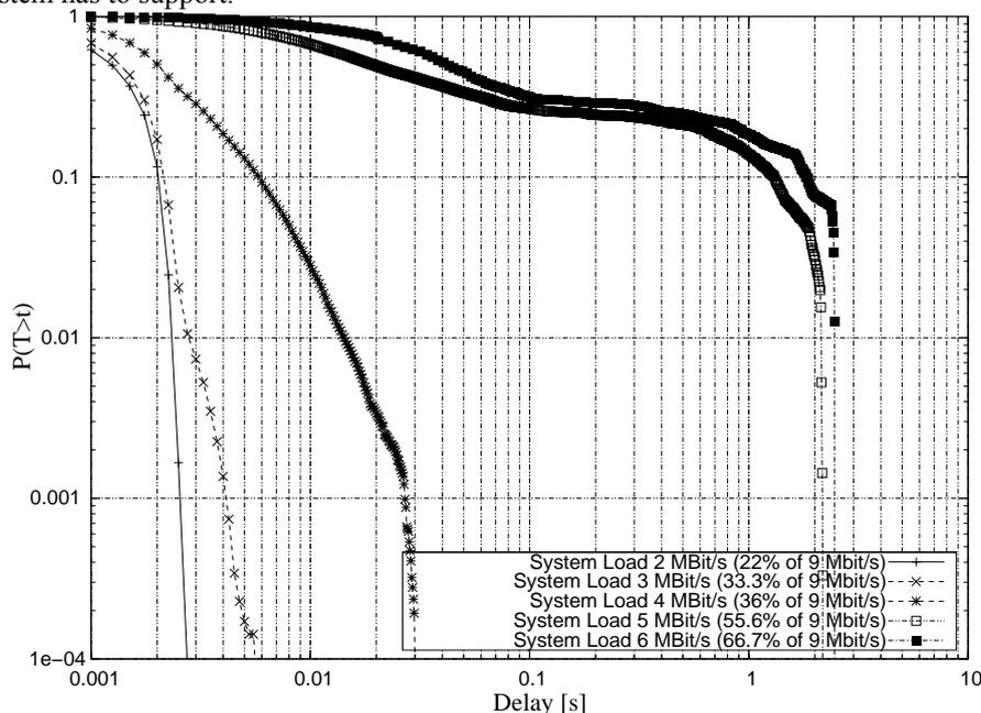
**Figure C-10: Pdf of downlink delay vs Load using Round Robin scheduling with FDT**
