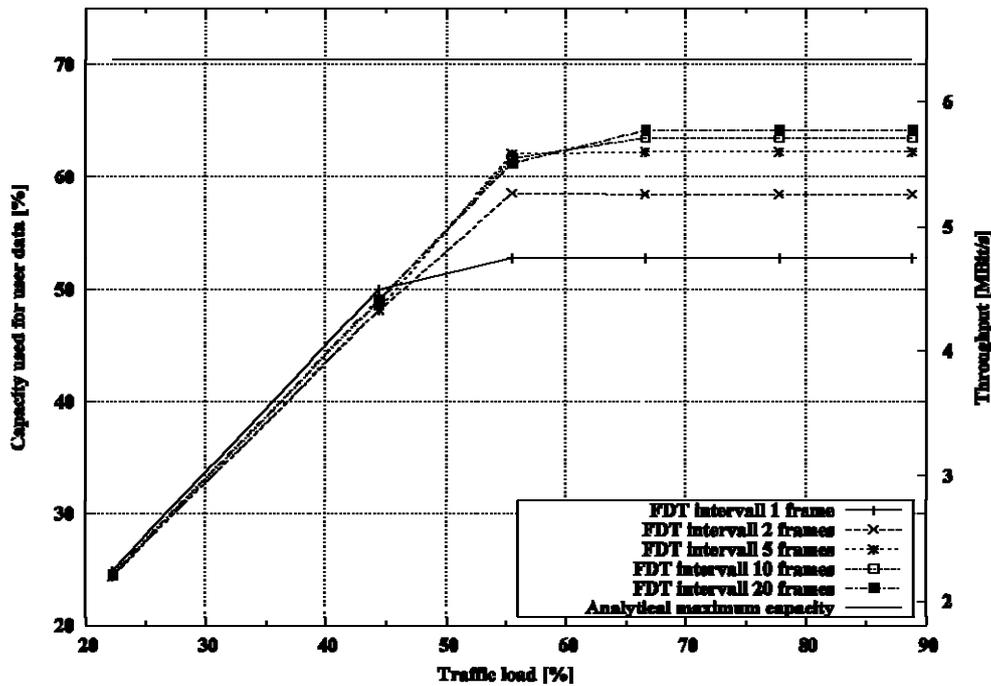
Figure C-8: Throughput vs. System Load depending on interval between changes of FD
