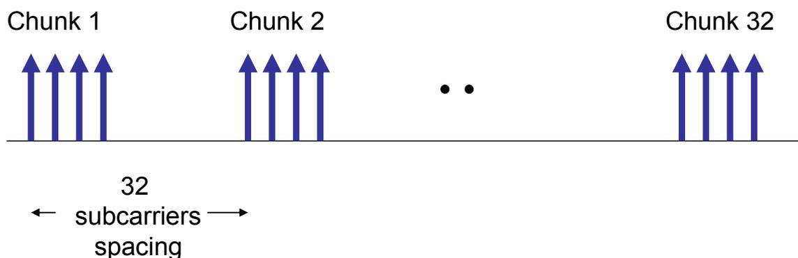
**Figure B-3: Frequency domain illustration of a signal with 128 subcarriers and chunk width=4, with chunks spaced at 32-subcarrier intervals.**
