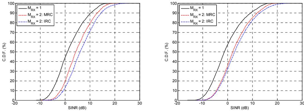
**Figure A-32: Post receiver SINR distributions in an interference limited network (left) and a noise limited network (right). The mobile terminals are equipped with different number of receive antennas (1, 2, and 4) and MRC or IRC is used.**
