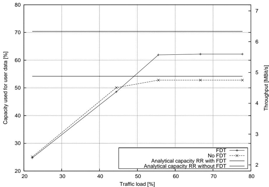
**Figure C-11: Throughput vs Load using Round Robin scheduling with and without FDT**
