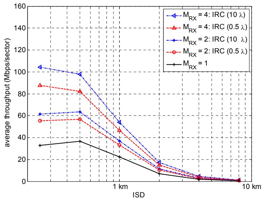
**Figure A-37: Average sector throughput as a function of the inter-site distance for different number of receive antennas (1, 2, and 4) and for different antenna separations (0.5 and 10 wavelengths). IRC is the used combining scheme.**
