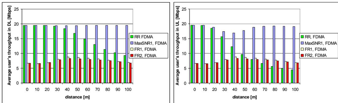
Figure A-19. Comparison of average user’s throughput for different schedulers, 40 allocated users
