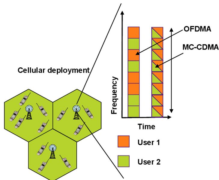
**Figure 4-1: Illustration of multiple access schemes. The TDMA/OFDMA scheme (left-hand alternative) represents exclusive allocation of chunk layers to flows.**
