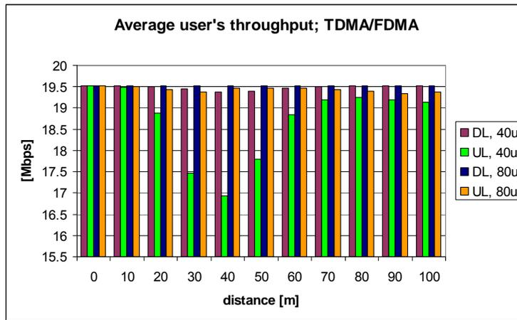
Figure A-18 Average user’s throughput vs. distance for the MaxSNR1 scheduler, 40 and 80 allocated users
