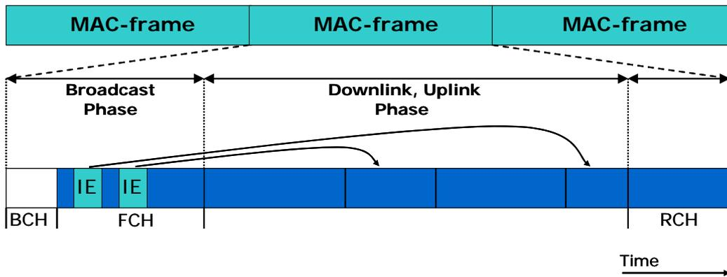
**Figure C-1: Basic MAC Frame structure**
