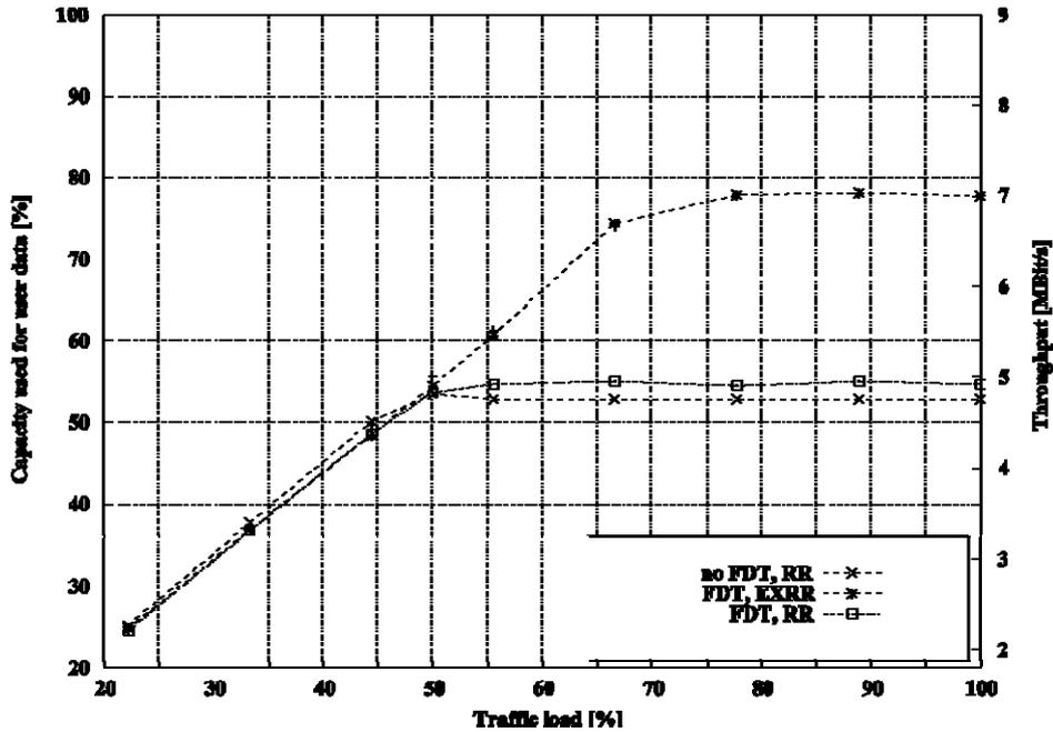
Figure C-12: Throughput vs. System Load depending on scheduling algorithm
