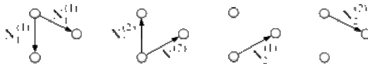
Figure 4-79: Distributed coding from [179]. Communication takes place in four phases. N_1^{(k)} denote the systematic bits of user k , and N_2^{(k)} are the corresponding redundancy bits. The drawing depicts the scenario where both terminals can decode their partner's systematic bits N_1 , thus being able to compute the corresponding N_2 bits and sending them in phase 2.
