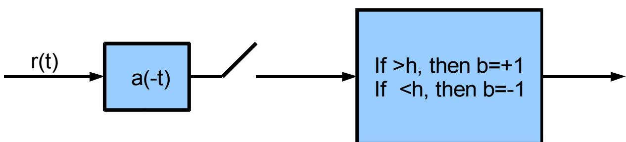
Determine the threshold  $h$  such that the receiver is a ML receiver. Compute the probability of bit error if  $p = 0.8$ .
